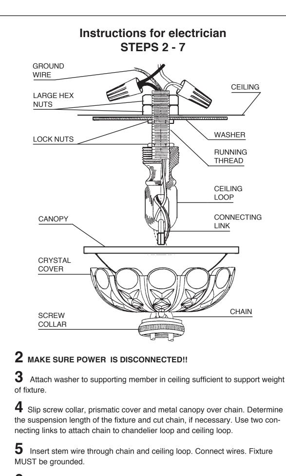
**6** Check distance from ceiling to loop to assure canopy assembly will be flush against ceiling.
