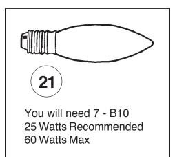
Install bulbs and be sure to test fixture BEFORE trimming.
