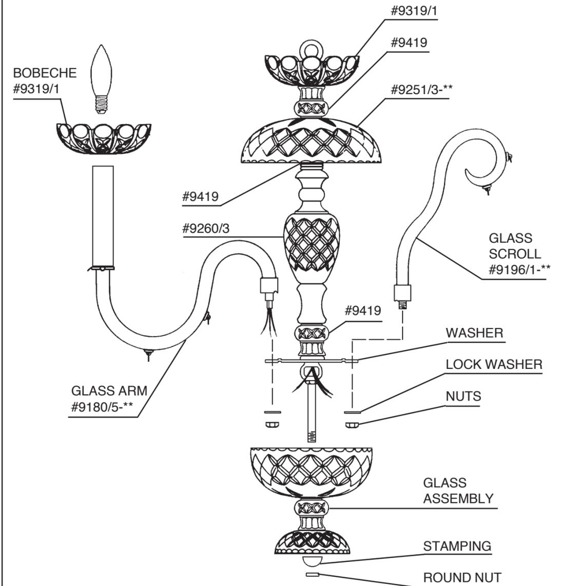
**8** Install arms and scrolls into washer. Line up holes in arms and scrolls with dimple in washer. Use lock washer and nut to secure arms and scrolls in place. **NOTE: Alternate arms and scrolls.**
