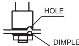
**5** Connect the wires of the wall bracket to the power wires of the outlet box, guide wall bracket over screw "A" and secure with threaded half ball supplied. NOTE: Fixture MUST be grounded.
