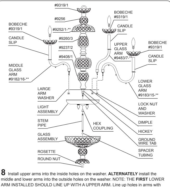
middle and lower arms into the outside holes on the washer. NOTE: THE FIRST LOWER ARM INSTALLED SHOULD LINE UP WITH A UPPER ARM. Line up holes in arms with dimple in washer. Use lock washer and nut to secure arms in place. Unscrew nut on nipple, place ground wire tab over nipple, secure with nut.
