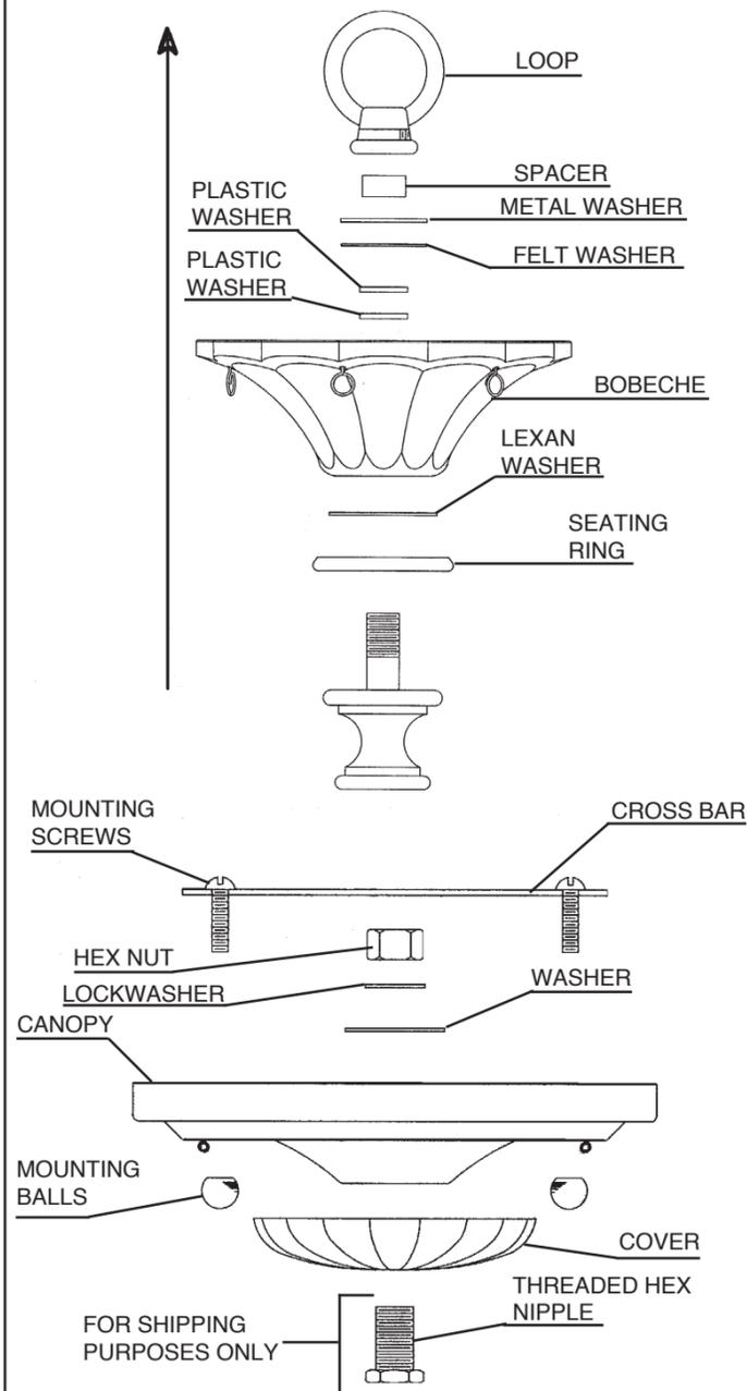
**3** Remove set screw from loop with tool provided. Remove all component parts from loop to seating ring. Remove threaded hex nipple and nut from assembled canopy. Run wires up through cover, canopy and component parts and tighten hex nut.
