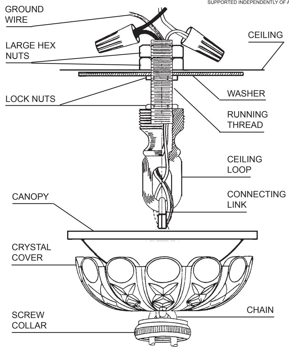
**WARNING:** THIS LUMINAIRE MUST BE MOUNTED OR SUPPORTED INDEPENDENTLY OF AN OUTLET BOX.
