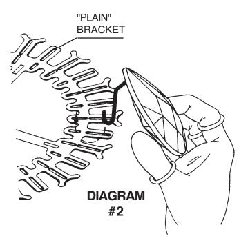
Position the crystal above the "plain" bracket so that the end of the hook enters the slot, gently push toward the center of the fixture and raise the crystal making sure that the end of the hook comes up through the inner slot, in line with the outer slot
