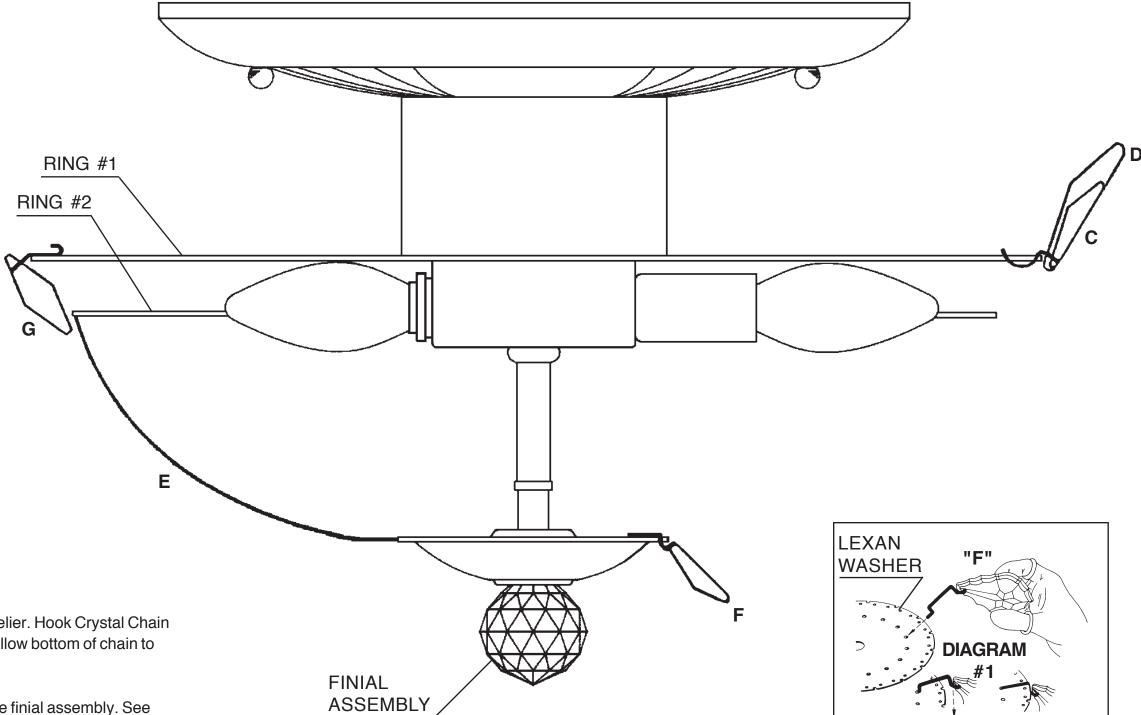
**7** Screw finial assembly onto bottom of chandelier. Hook Crystal Chain "E" (large crystal towards top) into the ring #2. Allow bottom of chain to hang freely.
