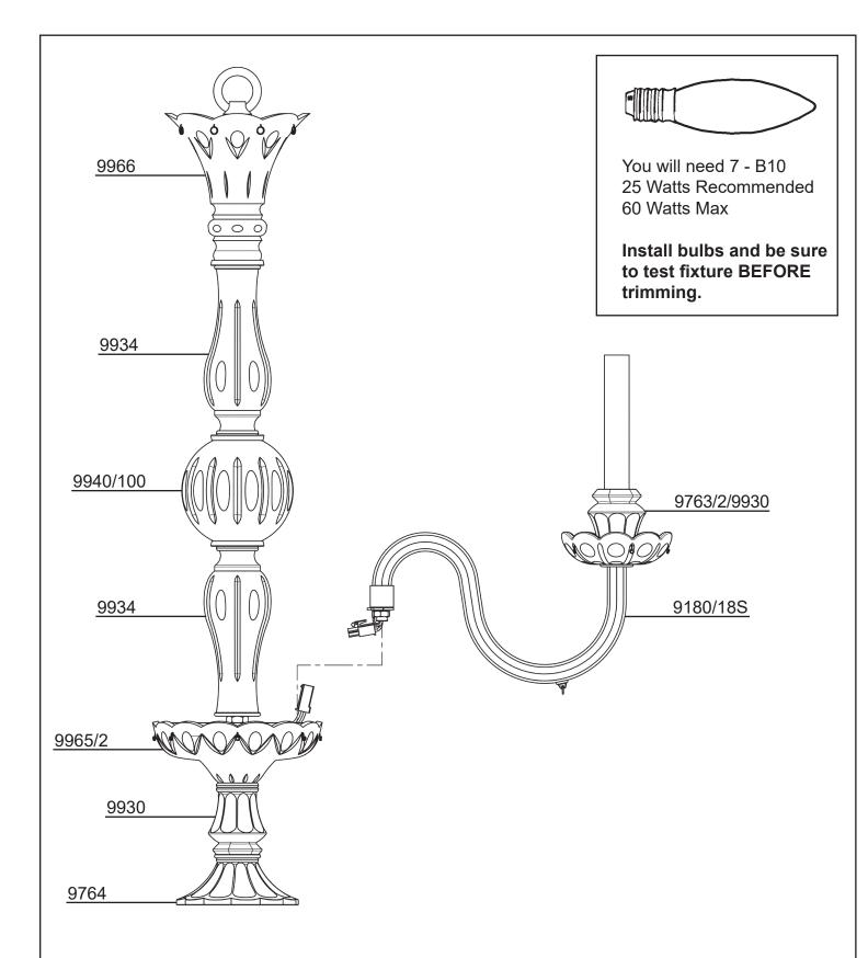
**20** Connect arm wires using plug-in connectors. See detailed illustration.
