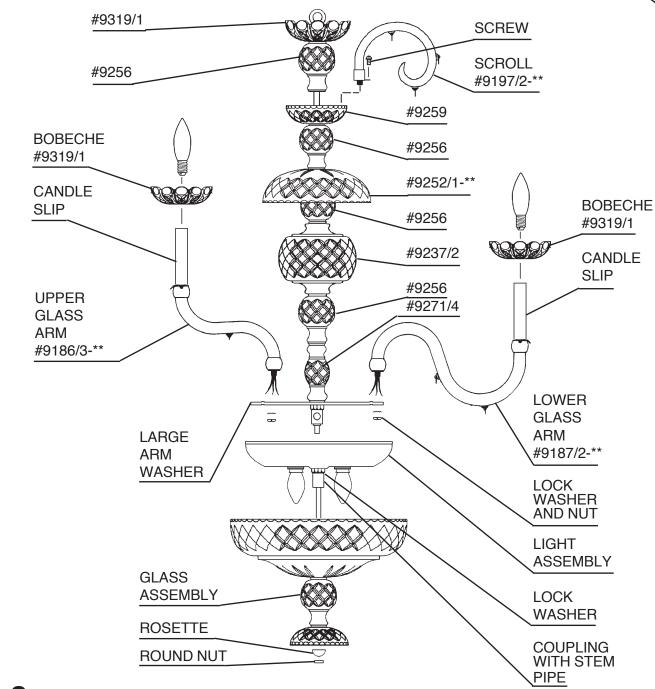
8 Install scrolls into washer with screws provided. Install arms into large arm washer. Line up holes in arms with dimple in washer. Use lock washer and nut to secure arms in place. NOTE: 6 Upper arms into inside diameter holes and 12 lower arms into outside diameter holes. Connect bare ground wires in each arm to bare ground wire in center column. Use electrical tape to secure wire nuts. NO MORE THAN 5 - WIRES PER WIRE NUT. Sufficient quantities of jumper wires and wire nuts are provided.
