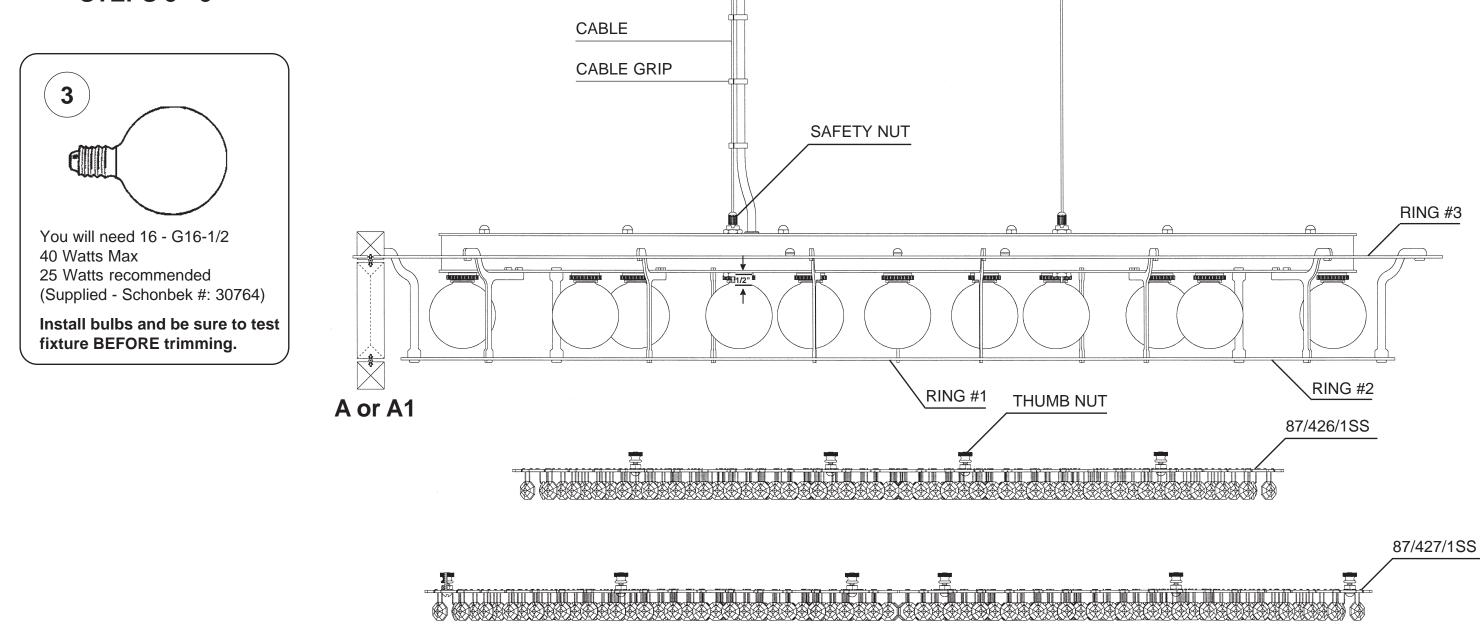
**4** Install two bottom crystal grids with twenty thumb nuts (already screwed onto grids) to bottom of rings #1 & #2.
