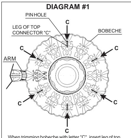
When trimming bobeche with letter "C", insert leg of top connector into pin hole from under bobeche. Hang in every other pin hole starting on either side of the arm (refer to Diagram #1)
